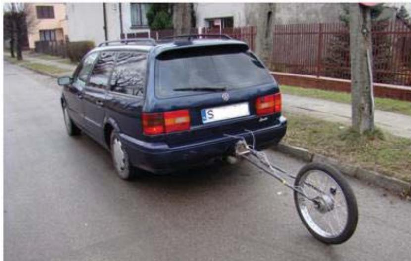
*Fig. 5. Measuring trolley used for the road tests*
